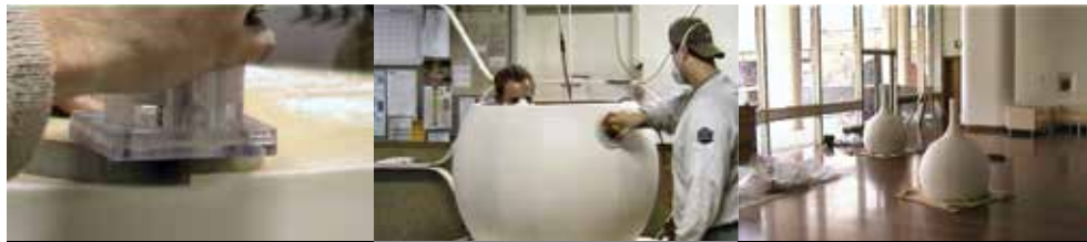
Final trimming of the shell Final sanding of the shell Assembly of 2 halves of a shell
