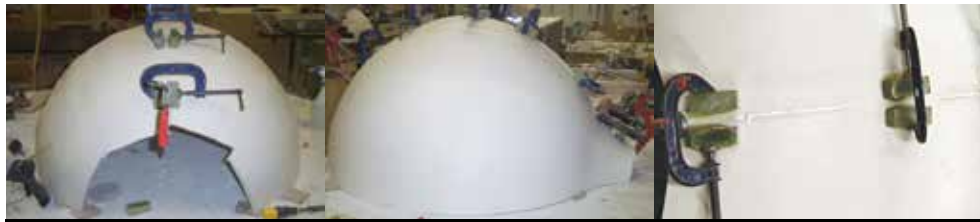
Assembly of 2 quarter pieces to half a shell
